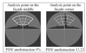
Figure 3: Uniform scenario sky obstruction projection with the point analysis on the façade middle and façade corner
